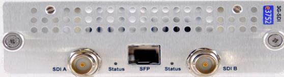
The SFP (Small Form-Factor Pluggable) interface supports multiple modules enabling the encoder to stream full HD video from broadcast-quality sources, such as Optical SDI and ST2022-6 interfaces.
